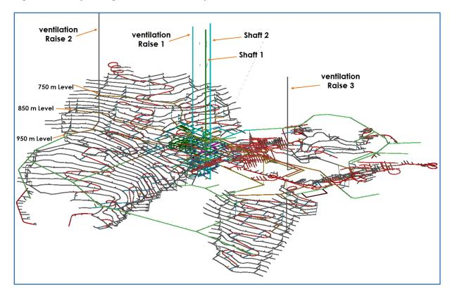
Figure 2 Platreef underground mine access layout.
